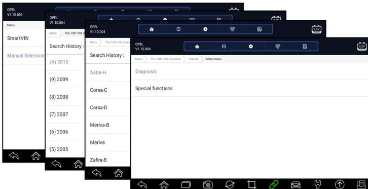
Figure 4-18 Sample Manual Vehicle Selection Screen
