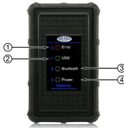
Figure 2-5 Front View of VCI dongle
