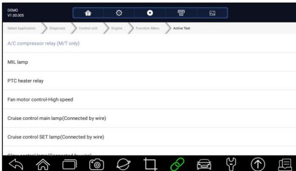
Figure 5-28 Sample Active Test Screen
